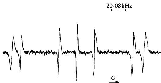
Fig. 3. An example of deuteron magnetic resonance spectrum from a single crystal of \text{Cu}(\text{NO}_3)_2 \cdot 2.5\text{D}_2\text{O} at a certain orientation about the symmetry axis.
